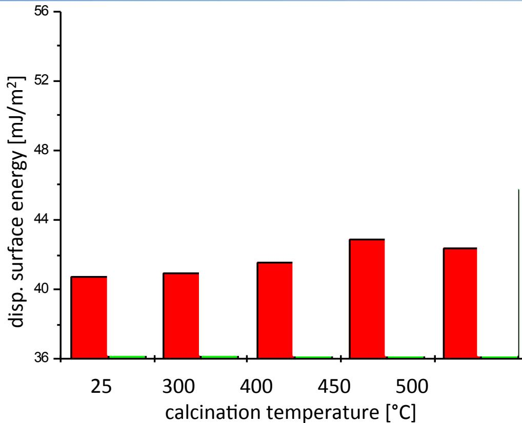
→ Porous glass beads exhibit a residual content of boron, that migrates to the surface during thermal treatment\*
