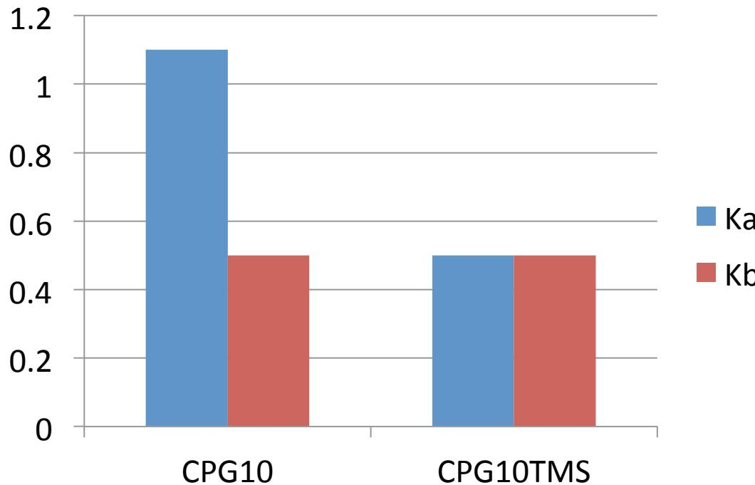
The surface modification with TMS groups has a significant impact on the potential of porous glass to interact with electron donating molecules (decreasing  $K_a$  value)
