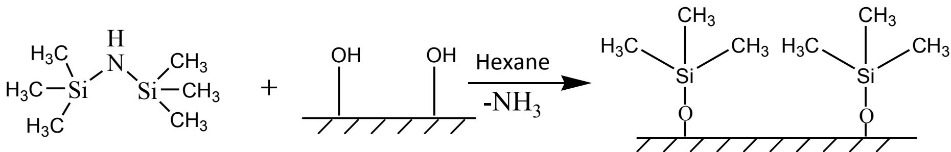
→ Generation of hydrophobic trimethylsilyl (TMS) groups onto the surface of the silicates
