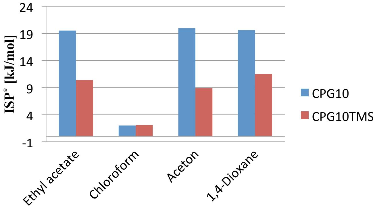
The surface modification has a strong impact onto the specific interactions. Generation of non-polar TMS groups causes a significant decrease of specific interaction parameter.
