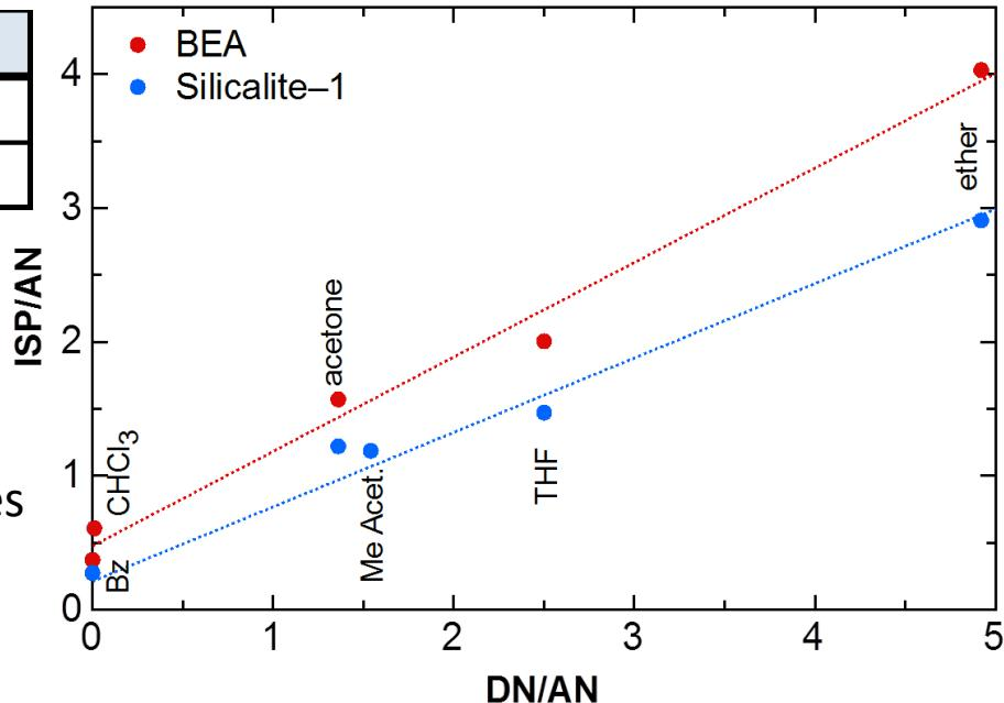
The two zeolites can be clearly differentiated by their electron donor and acceptor potential based on the retention times of known molecules
